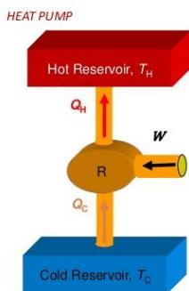
$$C.O.P. = \frac{Q_H}{Q_H - Q_C} = \frac{3.5 \text{ kW}}{3.5 \text{ kW} - 2.5 \text{ kW}} = 3.5$$
