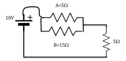
Parallel resistance is given by 1/R=1/5+1/15=>3.75 ohms +5 ohms in series, current = 1.14 Amps. voltage across parallel = 10- (1.14\*5)= 4.3 V; I=4.3/5= .86 amps
