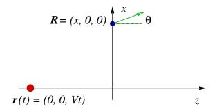
An object is moving with constant velocity V along the z-axis, i.e. along the curve
