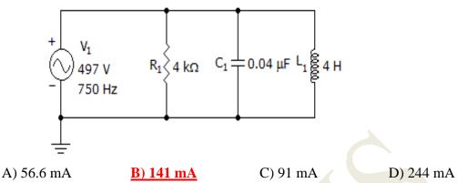
Since they are in parallel, the voltage over R, C and L is the same: the source voltage 497 V. The current through R is  $I_R=Vs/R$ , through C is  $I_C=Vs/Xc$ , and through L is  $I_L=Vs/X_L$ , where  $Xc=1/(2\pi f\cdot C)$  and  $X_L=2\pi f\cdot L$ . Thus  $Xc=5305\Omega$  and  $X_L=18850\Omega$ . This gives a current of  $I_R=12$  mA,  $I_C=9$  mA and  $I_L=3$  mA.
