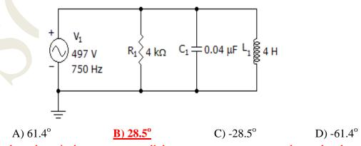
Since the voltage is the same across all the components, we want to know the phase angle the current makes to the voltage (see figure in problem 9). From above, the phase angle is  $\phi = \tan^{-1}((I_C\text{-}I_L)/I_R)$ , which is  $28.5^\circ$ . Hence net reactance of the circuit is capacitive, and the current will lead the voltage across the equivalent impedance of the circuit.
