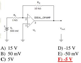
The op-amp will stabilize its output when there is no potential difference across its inputs. We have here that  $V_+=0$  V, so the potential at  $V_-$  must also = 0V. There is a potential difference across voltage divider of  $R_i=R_1$  and  $R_f=R_2$  of  $V_{in}$  -  $V_{out}$  that drives a current
