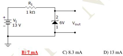
Since  $V_1 > V_{out}$ , the voltage across the Zener diode will be a constant 6 V. Thus, the voltage drop across the resistor,  $R_1$ , will be  $V_1$ - $V_z$ . Since the current through the resistor will also pass through the Zener, the current is driven by the voltage drop across  $R_1$ :  $I = (V_1 - V_2)/R = (13-6)V/1 k\Omega = 7 mA$  is the current through the diode.
