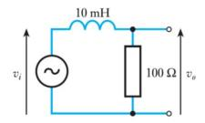
Using complex notation, the output voltage across the impedance divider is  $Vo = Vi*Z_R/(Z_R+Z_L)$ . Using complex notation, the response function is:
