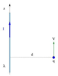
A particle of charge q is traveling in vacuum with velocity v parallel to an infinitely long wire of a constant uniform charge distribution  $\lambda > 0$  per unit length (see figure). The wire also carries a constant current I directed as shown in the figure. In this problem the gravitational force acting on the particle can be neglected.
