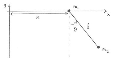
A pendulum system (see above) comprises two masses  $m_1$  and  $m_2$  where the first one acts as a frictionless sliding pivot along the x-axis for the latter mass.
