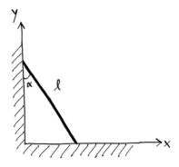
initial value  $\theta(0)=\alpha$ . The initial angular velocity is  $\dot{\theta}(0)=0$ . The plate itself is homogeneous and its principal moment of inertia around the perpendicular principal z-axis and the center-of-mass is  $I_Z=\frac{m\ell^2}{12}$ . [Answer: The equation of motion will be  $\ddot{\theta}=3g/(2\ell)sin\theta$ .]
