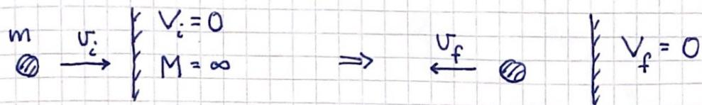
$$v_f = \frac{M}{m+M} \cdot \left\{ 0 + v_i \cdot \frac{m-M}{M} \right\} \stackrel{m \ll M}{=} -v_i$$
