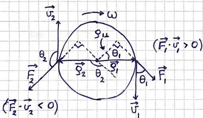
$$\begin{aligned} P &= \sum_i \vec{F}_i \cdot \vec{v}_i \\ &= \sum_i F_i v_i \cos \theta_i \\ &= \left\{ \sum_i F_i s_i \cos \theta_i \right\} \cdot \omega \\ &= \underbrace{\left\{ \sum_i F_i s_{i\perp} \right\}}_{= \tau} \cdot \omega \end{aligned}$$
